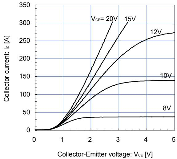
Collector current vs. Collector-Emittter voltage (typ.)
