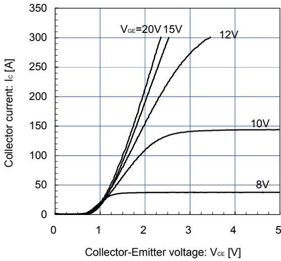
Collector current vs. Collector-Emittter voltage (typ.)
