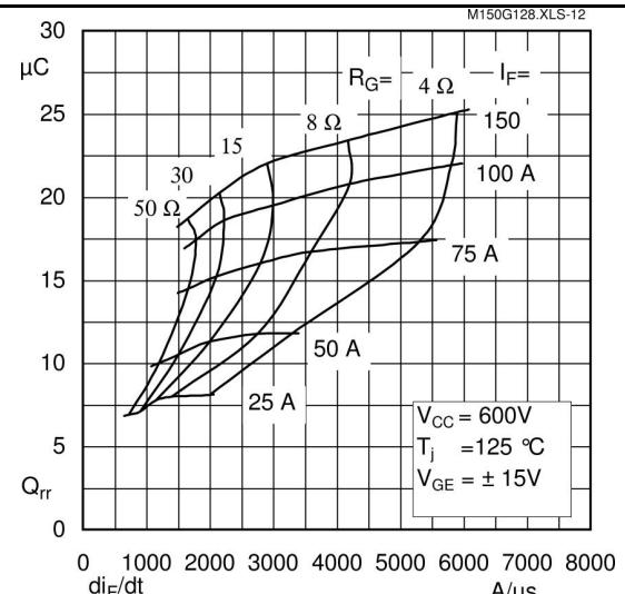
Fig. 12 Typ. CAL diode peak reverse recovery charge
