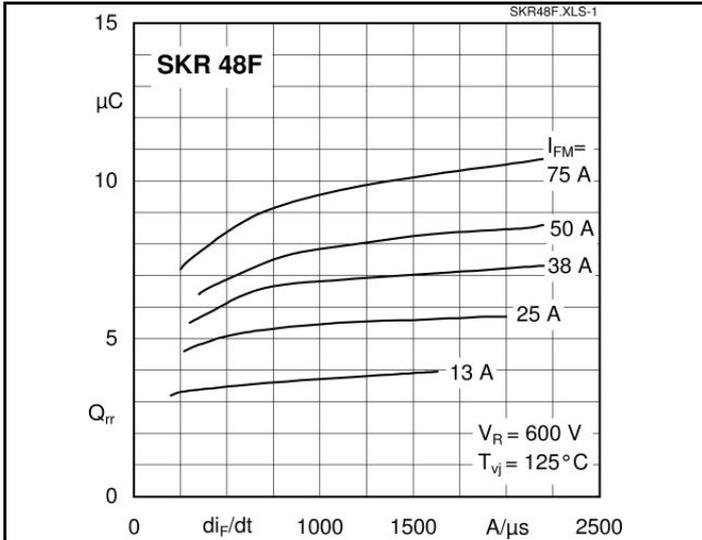
Fig. 1 Typ. recovery charge vs. current decrease
