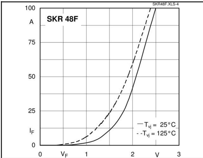
Fig. 4 Forward characteristics
