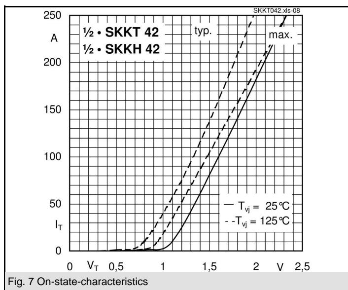
Fig. 7 On-state-characteristics
