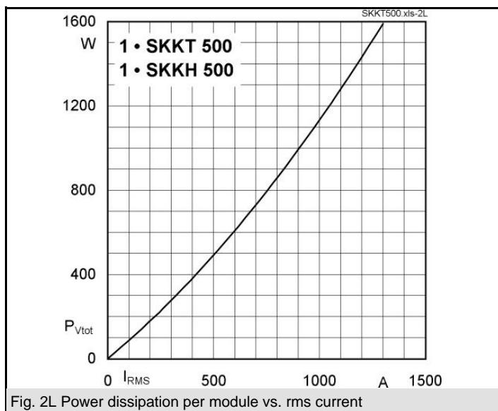
Fig. 2L Power dissipation per module vs. rms current
