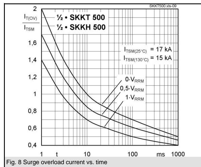
Fig. 8 Surge overload current vs. time
