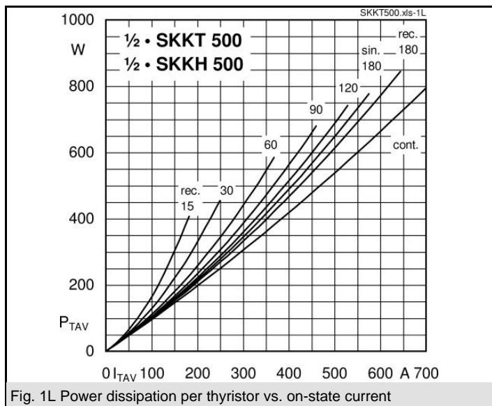
Fig. 1L Power dissipation per thyristor vs. on-state current
