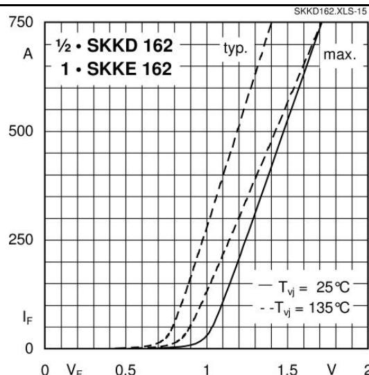
Fig. 15 Forward characteristics
