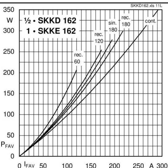
Fig. 11L Power dissipation per diode vs. forward current
