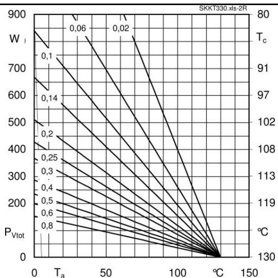
Fig. 2R Power dissipation per module vs. case temp.
