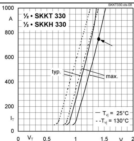
Fig. 7 On-state characteristics
