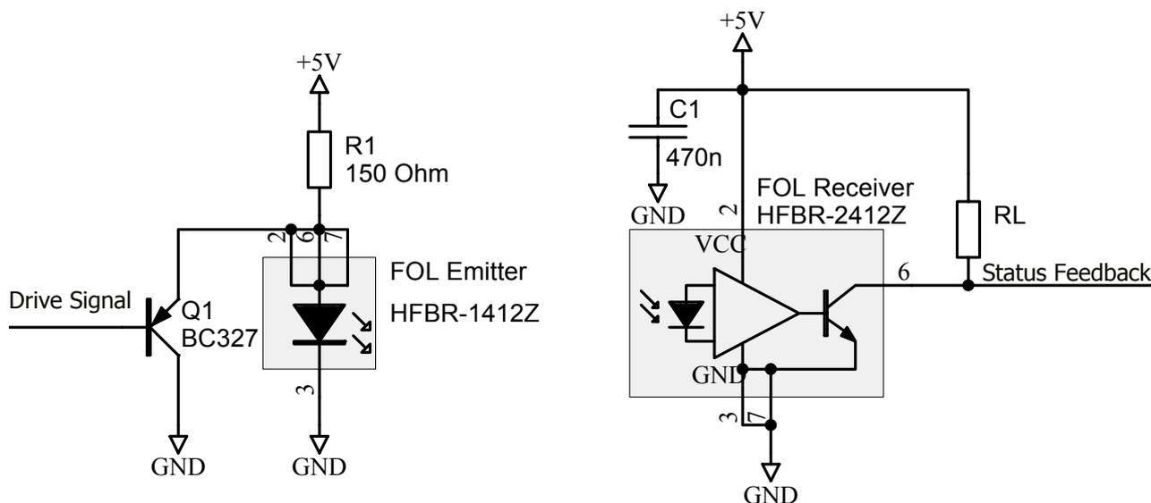
Fig. 13 Recommended circuitry for the "ST" fiber-optic links (1SP0635S)
