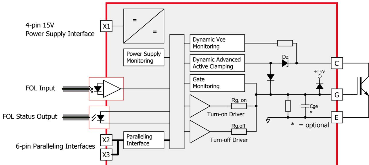
Fig. 2 Basic schematic of the 1SP0635V and 1SP0635S drivers
