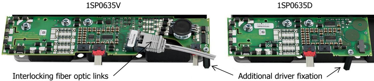
Fig. 19 Additional measures for fixing the drivers (1SP0635V/1SP0635S left, 1SP0635D right) as well as the relevant version of interlocking fiber-optic links for the 1SP0635V
