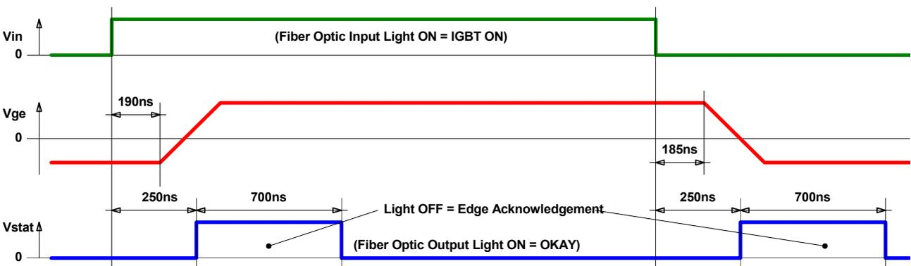
Fig. 8 Driver behavior and status feedback in normal operation
