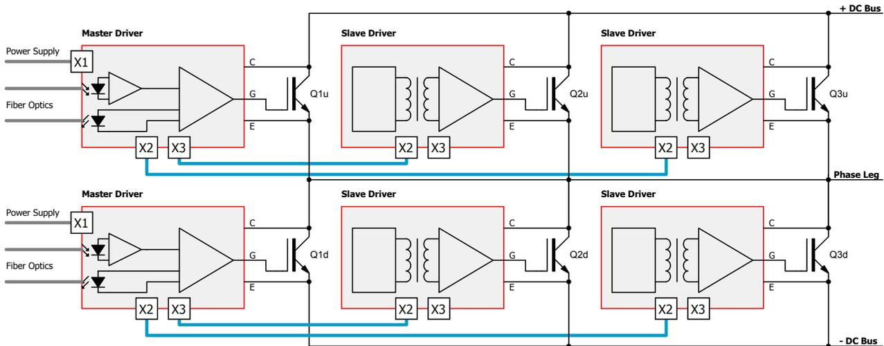
Fig. 4 Principle of parallel connection of 1SP0635 drivers with one master and two slaves in a half-bridge configuration (example)
