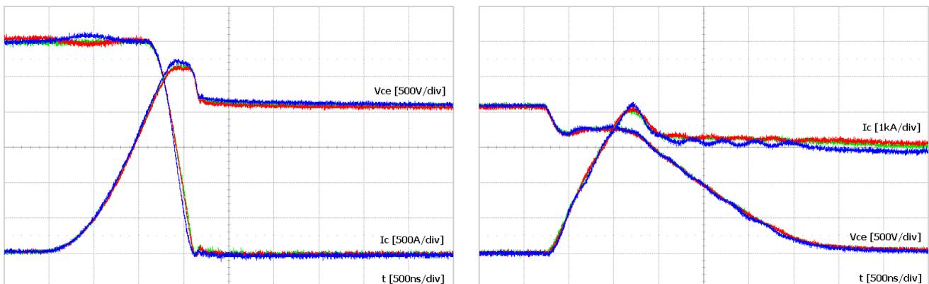
Fig. 16 Turn-off (left) and turn-on (right) behavior of three 1500A/3300V IGBT modules in parallel connection at a DC-link voltage of 2200V and a collector current of 3000A each
