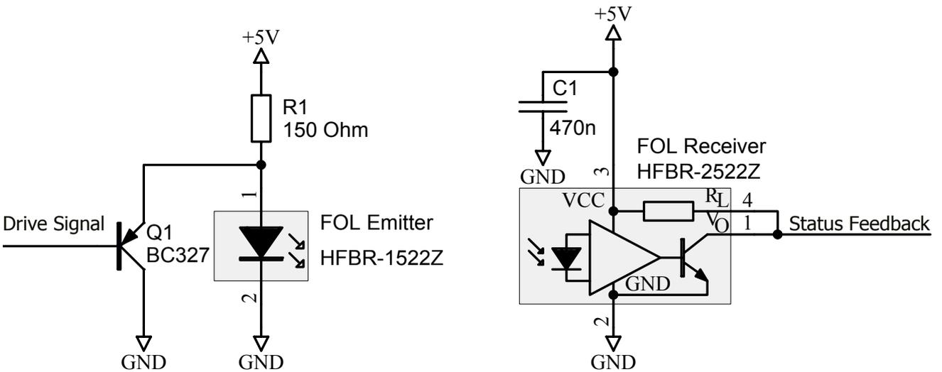
Fig. 12 Recommended circuitry for the “versatile” fiber-optic links (1SP0635V)
