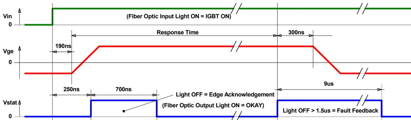
Fig. 9 Driver behavior and status feedback in the short-circuit condition
