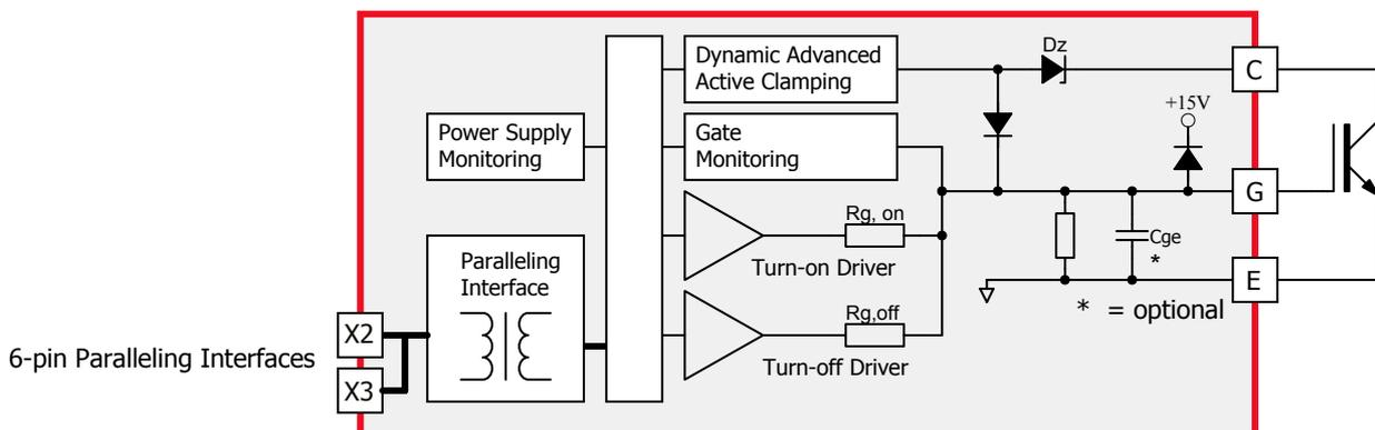
Fig. 3 Basic schematic of the 1SP0635D drivers
