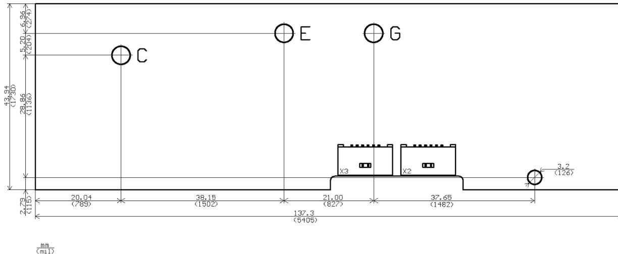
Maximum driver height: 6mm measured from the bottom layer
