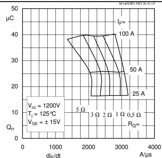
Fig. 12 Typ. CAL diode recovered charge
