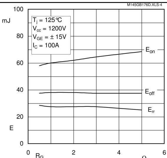
Fig. 4 Typ. turn-on /-off energy =  $f(R_G)$
