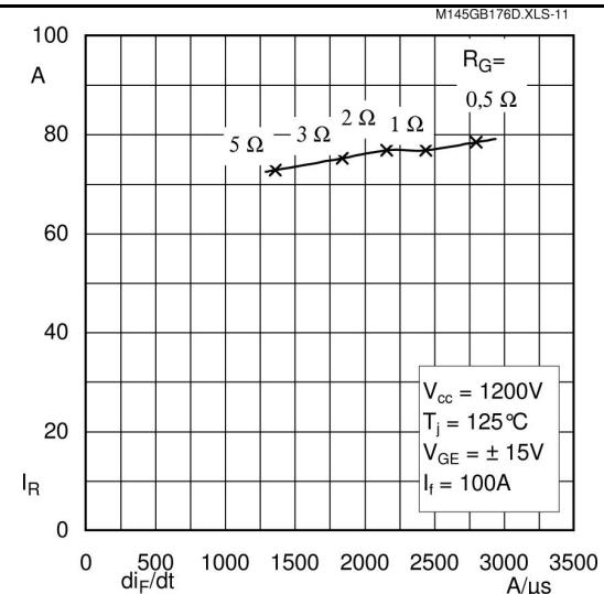
Fig. 11 Typ. CAL diode peak reverse recovery current
