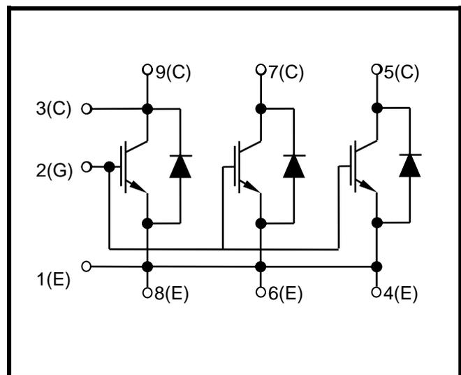
Fig. 1 Circuit configuration
