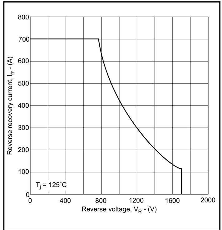
Fig. 8 Diode reverse bias safe operating area
