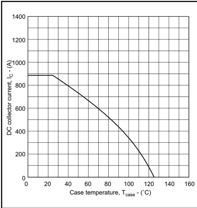
**Fig. 11 DC current rating vs case temperature**
