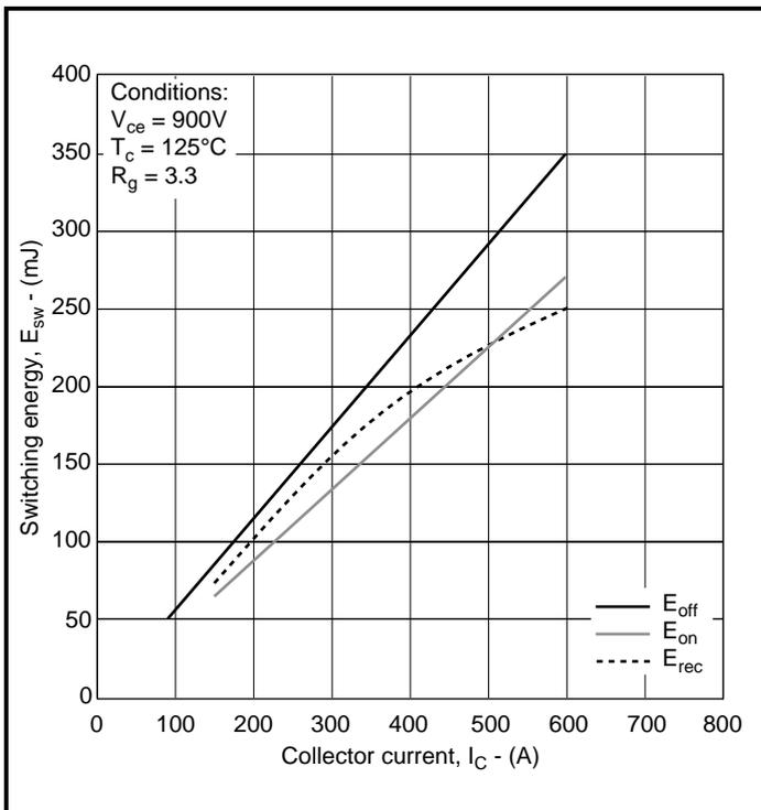
**Fig. 5 Typical switching energy vs collector current**
