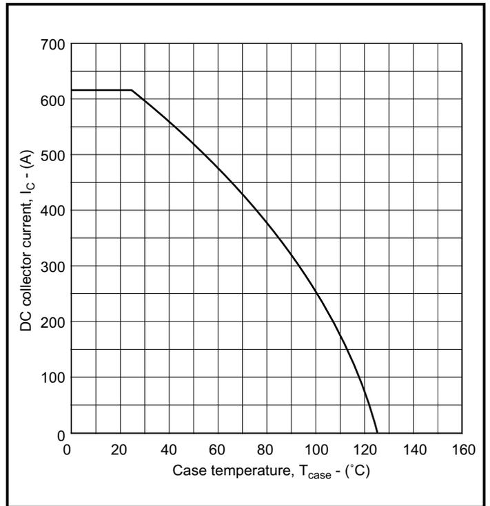
Fig. 14 DC current rating vs case temperature
