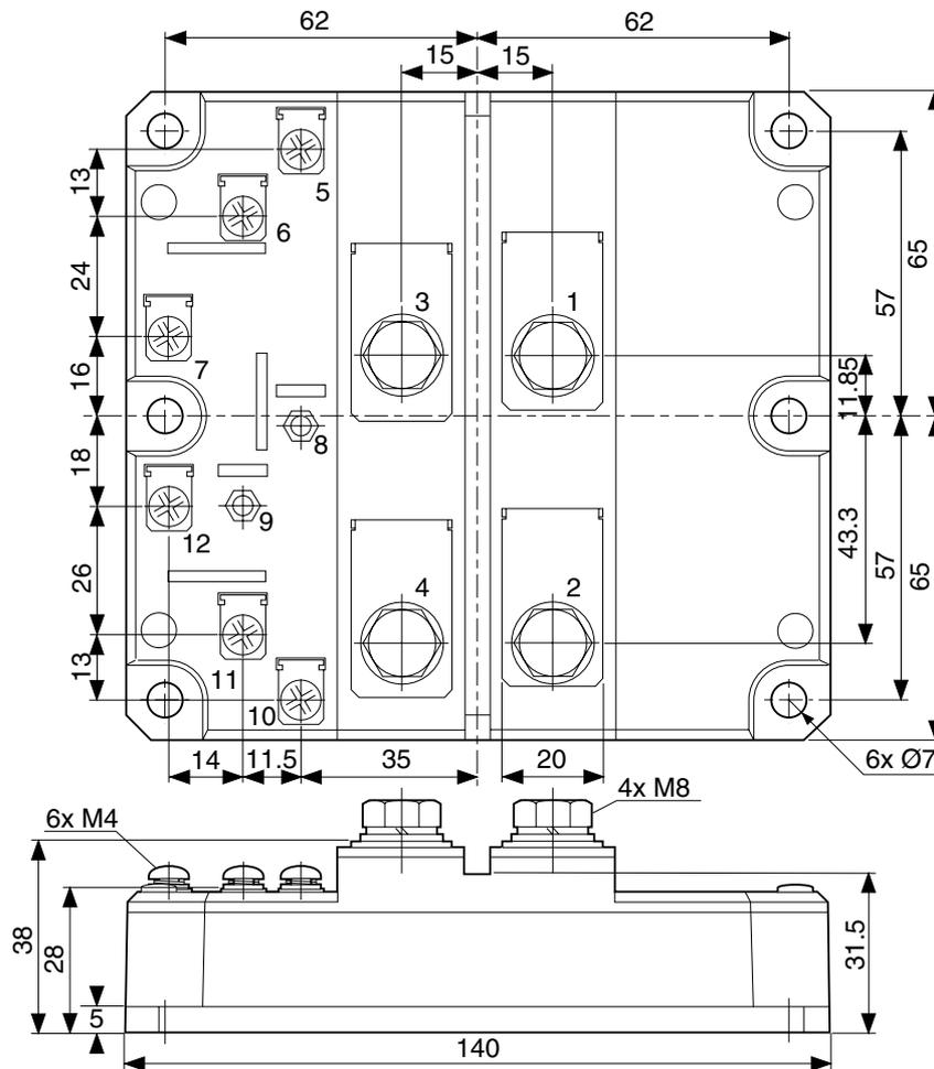
Main Terminal screw plastic hole depth (M8) =  $16.8 \pm 0.3$
