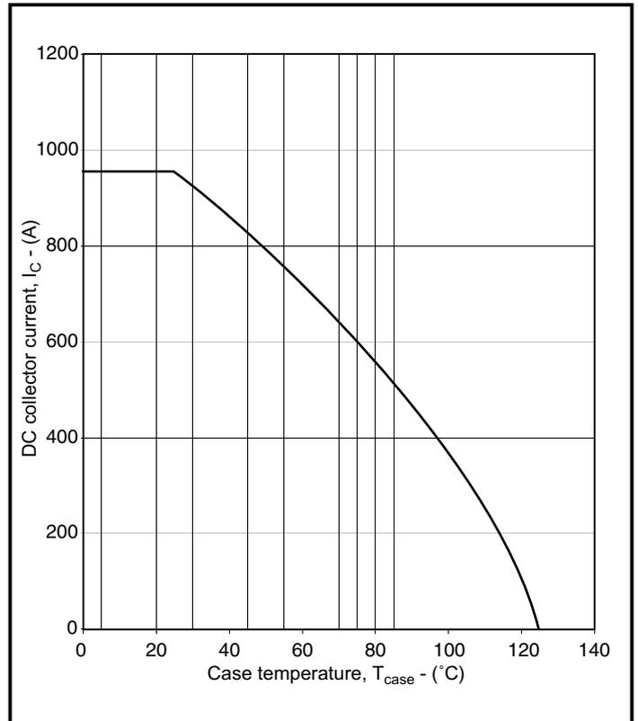
**Fig. 10 DC current rating vs case temperature**
