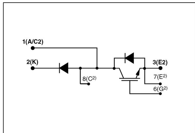
Fig. 1 Chopper circuit diagram
