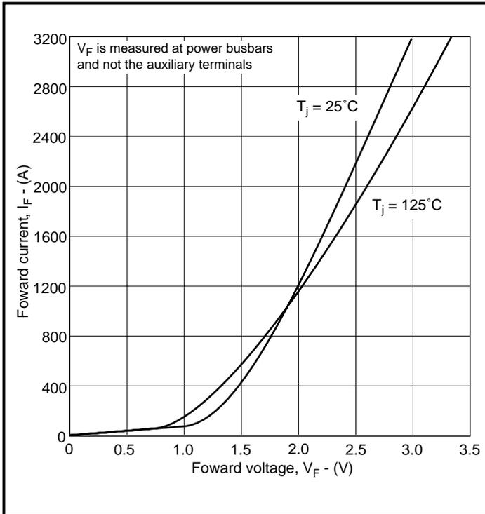
**Fig. 7 Diode typical forward characteristics**
