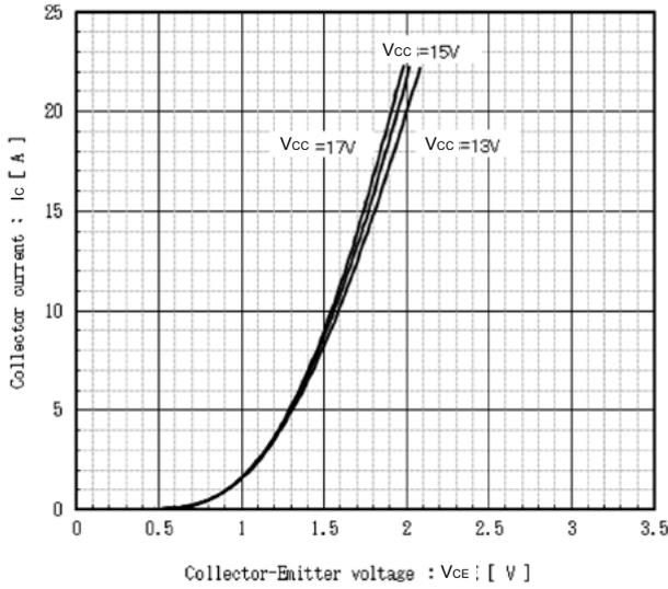
Collector current vs. Collector-Emittter voltage
