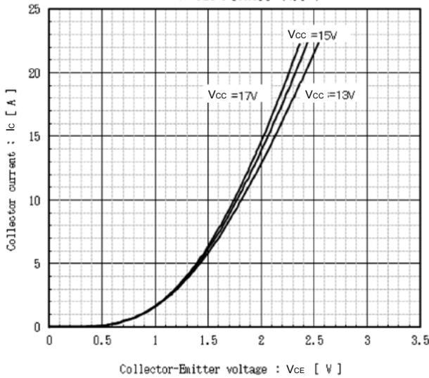
Collector current vs. Collector-Emittter voltage
