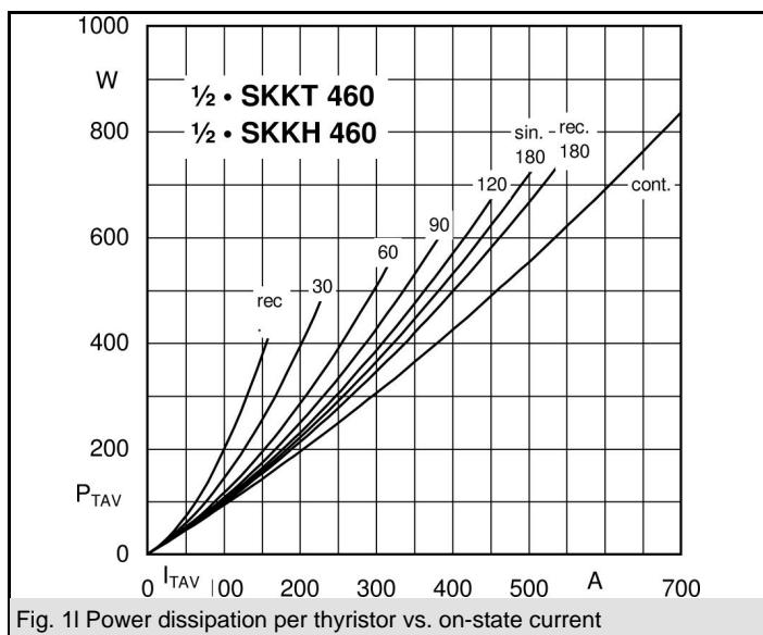
Fig. 1I Power dissipation per thyristor vs. on-state current
