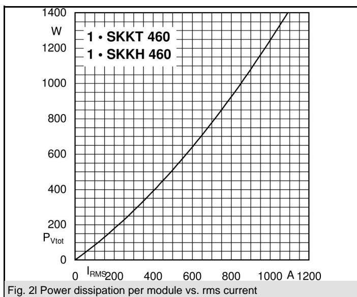
Fig. 2I Power dissipation per module vs. rms current
