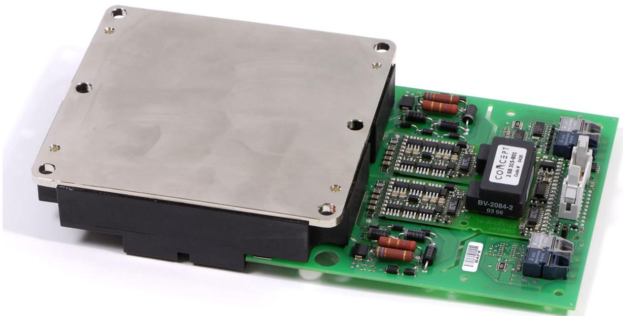
*Fig. 1a 2SB315B screwed onto a 130mmx140mm IGBT module (bottom view)*
