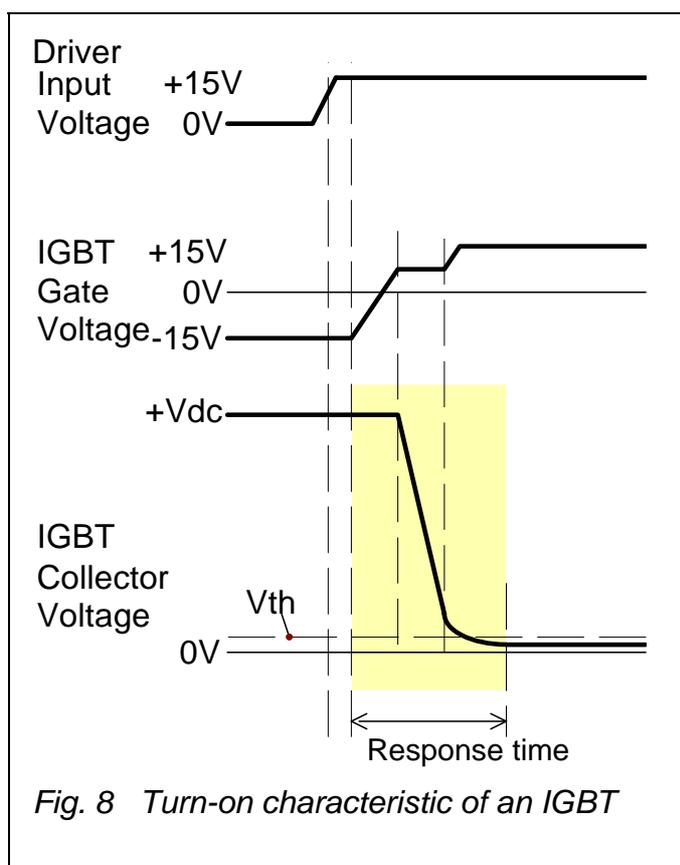
Each channel of a SCALE driver is equipped with a  $V_{ce}$ -monitoring circuit. The circuit is inactive during the response time applied to ensure that the IGBT is fully turned on (see Fig. 8).
