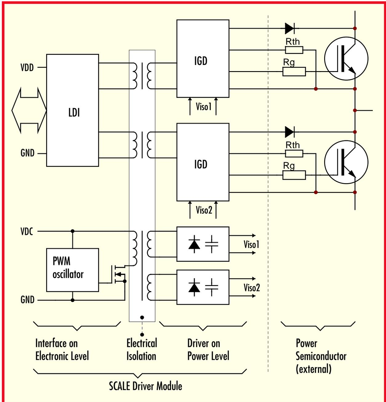
Fig. 1 Block diagram of the 2SD106A
