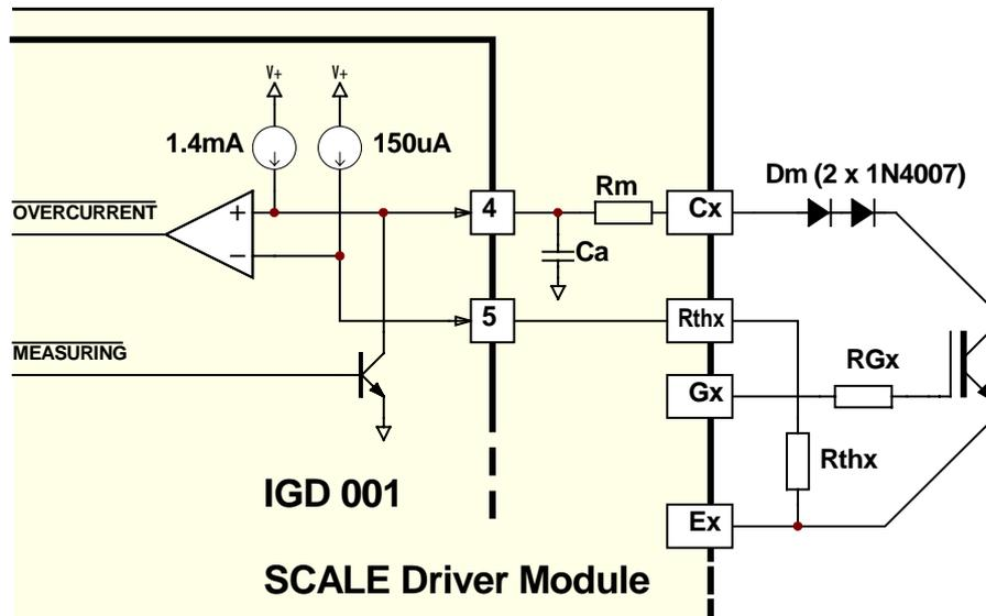
The 2SD106A dual driver has a collector-sense circuit to protect the power semiconductors. It is shown in Fig. 4
