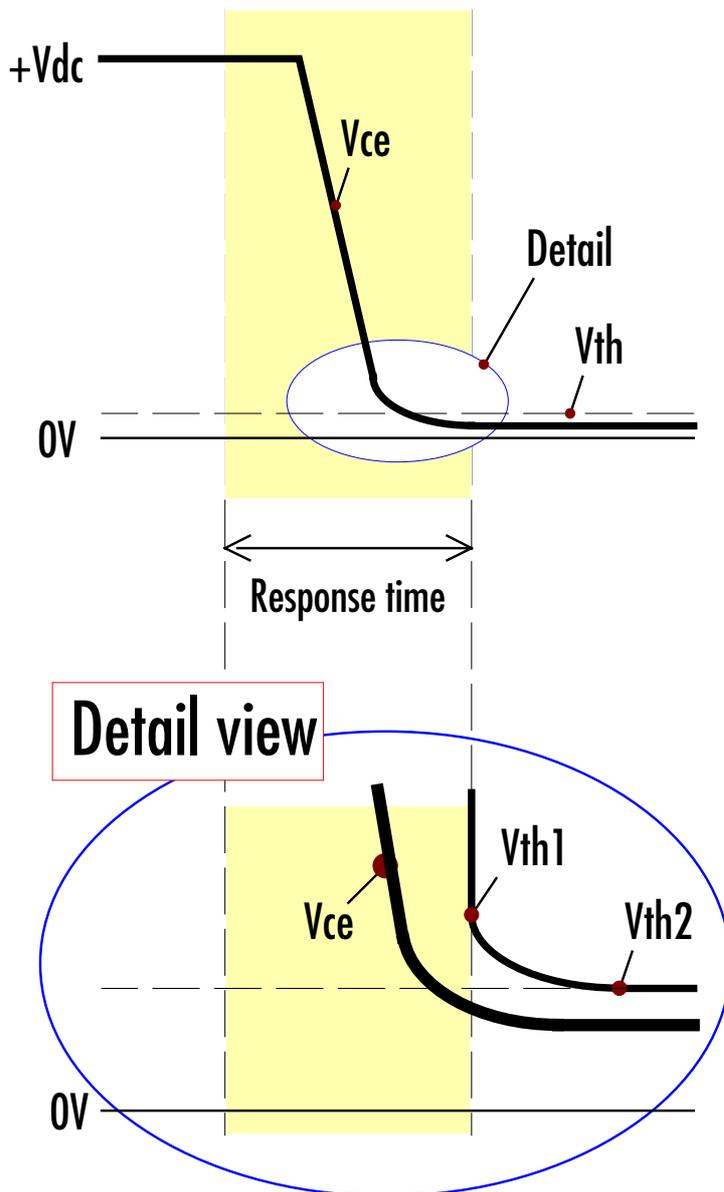
Fig. 5 Collector-sense voltage curve
