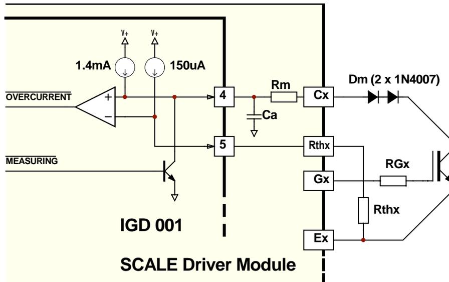
The 2SD106AI-17 dual driver has a collector-sense circuit to protect the power semiconductors. It is shown in Fig. 4
