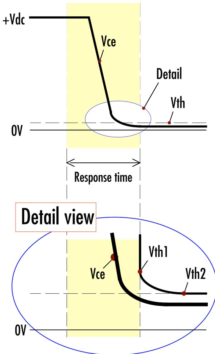
Fig. 5 Collector-sense voltage curve
