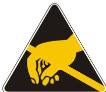
Any handling of IGBT modules or drivers is subject to the general specifications for protecting electrostatic-sensitive devices according to international standard IEC 747-1, Chapter IX or European standard EN 100015 (i.e. the workplace, tools, etc. must comply with these standards). **If these specifications are ignored, both IGBTs and drivers may be damaged.**
