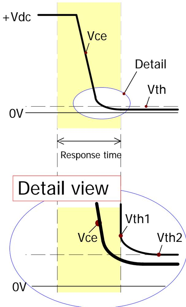
of the IGBTs, the SCALE drivers do not use a static reference voltage to compare the voltage at the collector. Instead, the reference is used as shown in Fig. 5.
