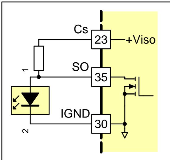
Fig. 8 Fiber-optic transmitter wiring
