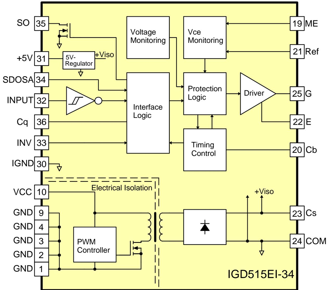
Fig. 1 Block and connection diagram of the IGD515EI-34
