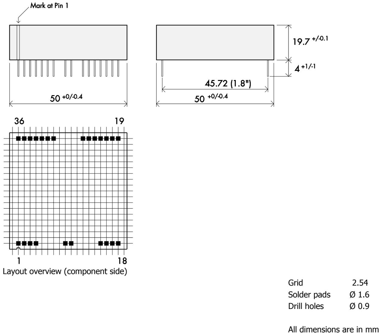
Fig. 2 Mechanical dimensions and printed circuit layout
