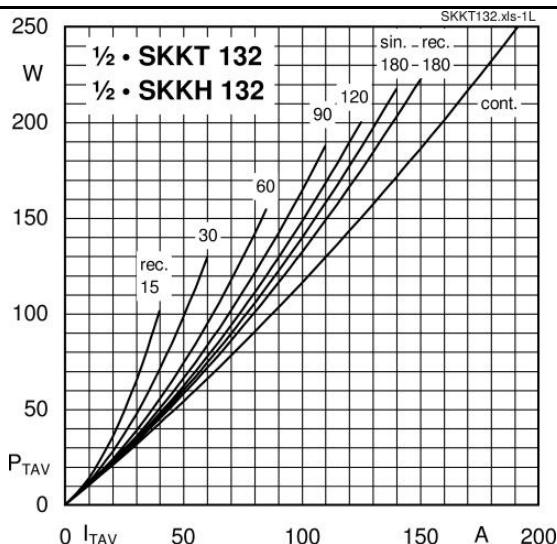
Fig. 1L Power dissipation per thyristor vs. on-state current
