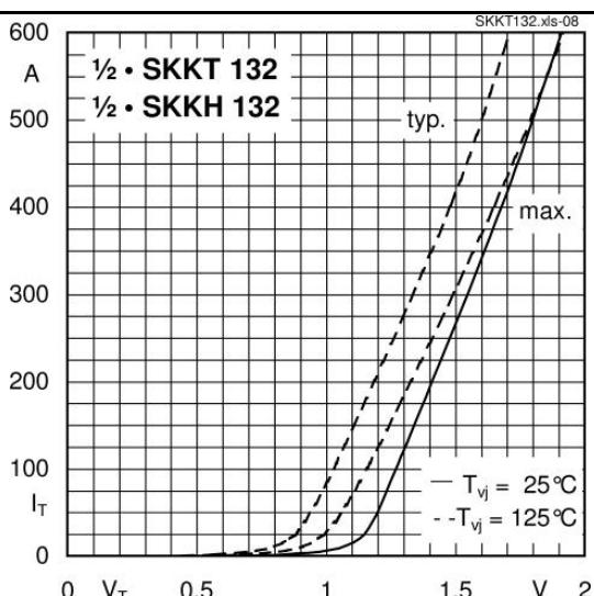
Fig. 7 On-state characteristics
