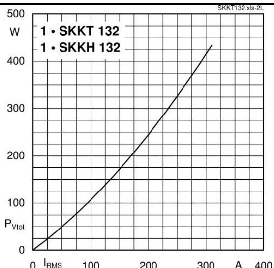
Fig. 2L Power dissipation per module vs. rms current
