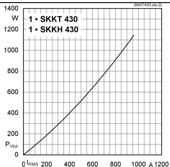
Fig. 2L Power dissipation per module vs. rms current
