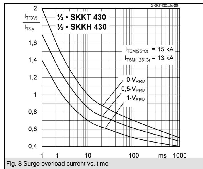
Fig. 8 Surge overload current vs. time
