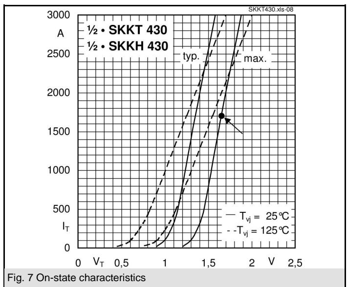
Fig. 7 On-state characteristics
