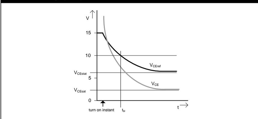
After  $t_{bl}$  has passed, the  $V_{CE}$  monitoring will be triggered as soon as  $V_{CE} > V_{CEref}$  and will turn off the IGBT. The error memory will be set, and the output PRIM\_HOLD\_OUT changes to the HIGH state. Possible failure modes are shown in the following pictures.
