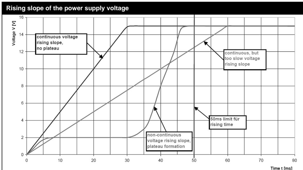
If the power supply is able to provide a higher current, a peak current will flow in the first instant to charge up the input capacitances on the driver. Its peak current value will be limited by the power supply and the effective impedances (e.g. distribution lines), only.
